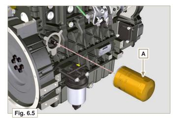
2 - Assembly and tighten the new oil filter cartridge A tightening it with torque wrench B (torque to 15 Nm).
